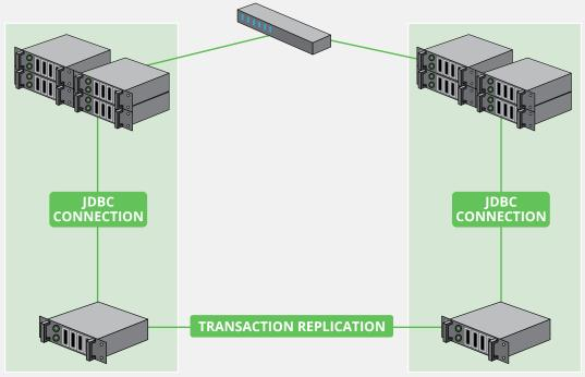
One or more Application Servers connected to the database server using standard JDBC connectivity.
